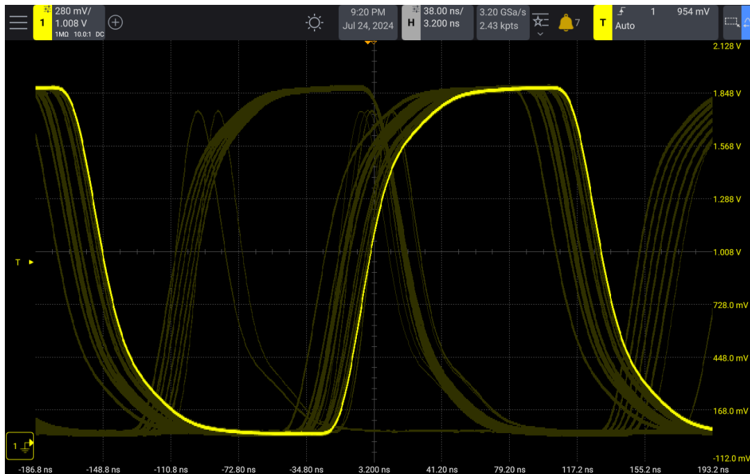
Figure 2. An update rate of 1.3 million waveforms per second easily captures infrequent glitches and jitter.
