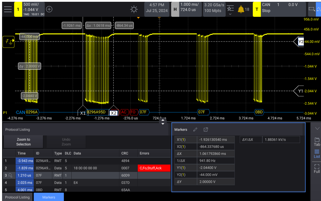
Figure 3. Hardware-based decoding captures and displays an infrequent CAN stuff bit error followed by an error frame.
