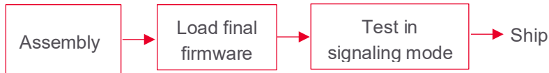
Figure 3. Streamlined test flow by testing in signaling mode with IOT8720 and IOT8740A
