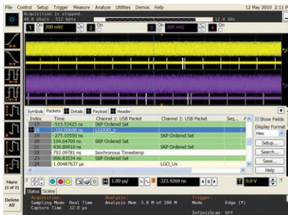
Isolate signal integrity problems from logic-level coding errors on bidirectional serial data streams.
