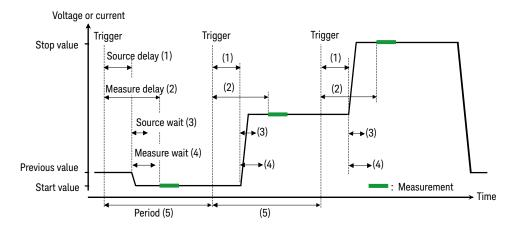
To set the delay time and the period, see "Trigger Parameters" on page 125. To set the wait time, see "Wait Control Dialog Box" on page 136. For more information about the trigger setup, see "Trigger Key Group" on page 140.
