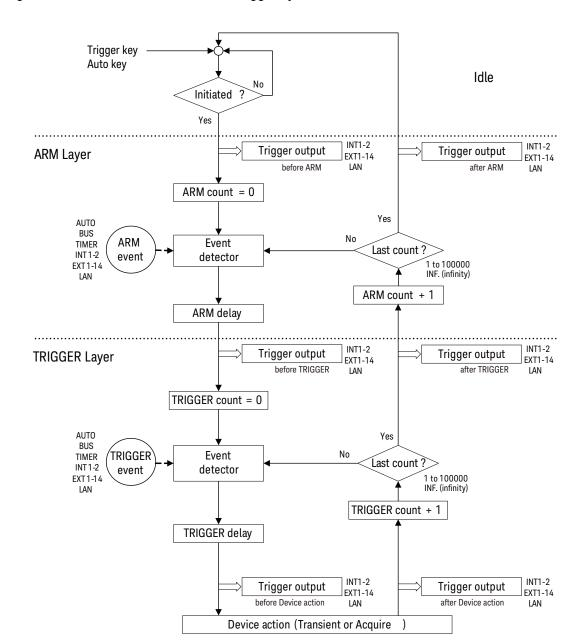
Figure 6-7 B2961B/B2962B Trigger System
