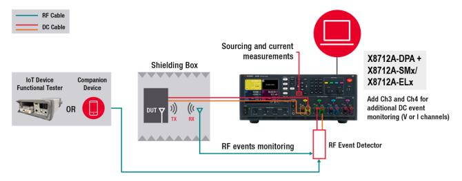
Figure 3. The X8712A synchronizes and correlates current consumption with RF/DC events
