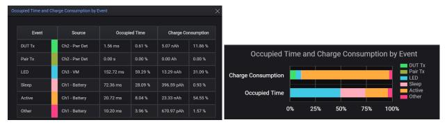
Figure 10. Obtain an RF or DC event's occupied time and charge consumption in %.
