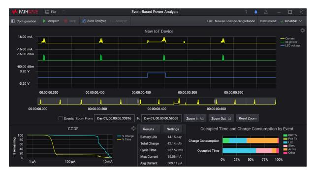
Figure 13. Battery life predicted based on four full operational cycles and 0.2-Ah battery capacity
