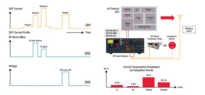
Figure 2. The X8712A Event-based Power Analysis Concept
