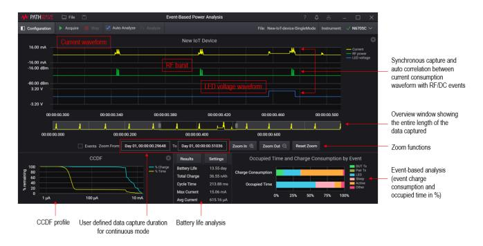
Figure 4. Overview of the KS833A2A Event-based Power Analysis Software
