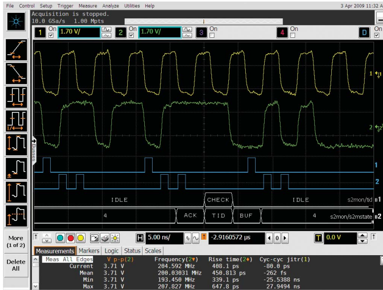
Use the MSO timing channels to evaluate control signal relationships and data buses up to 16 bits wide. Use symbols to more quickly interpret waveforms.
