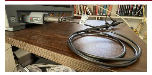
Above, you can see the PP0001A interfacing with an Infiniium oscilloscope via the PP0004A adapter. Below, you can see how the connection will look on future oscilloscopes, directly connected.
